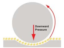
The shear strength of the fluid increases due to an increase in load or pressure of a surface and behaves as though it were stronger than the metal surface it acts against, thus causing the surface to deform.
