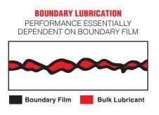
**Boundary Lubrication** is a condition in which the lubricant film becomes too thin to provide total surface separation. This may be due to excessive loading, low speeds or a change in the fluid's characteristics. In such cases, occasional metal-to-metal contact takes place between surfaces, and the surfaces are almost entirely dependent on the lubricant's additives to provide protection.
